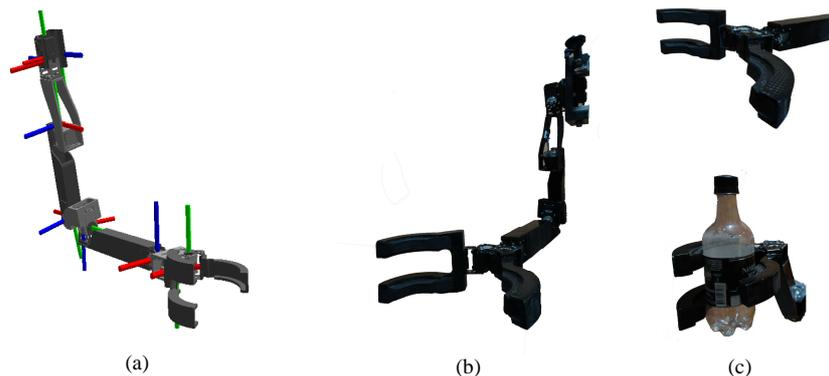
Figure 2. Bender's new arm. (a) Shows the Simulated right arm with the DOFs and the respective axes for every joint between the parts of the arm. (b) Real Right arm in a manipulation pose. (c) Different views of the real right hand gripper in a manipulate action.
