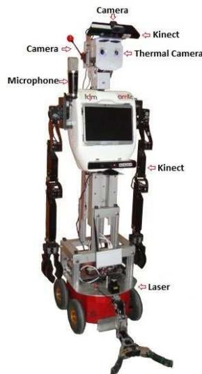
Figure 1. Bender, the official robot of the UChile HomeBreakers team.
