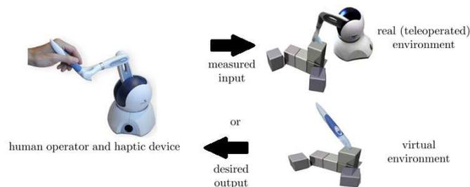
Figure 4. The haptic loop of a generic haptic interface.
