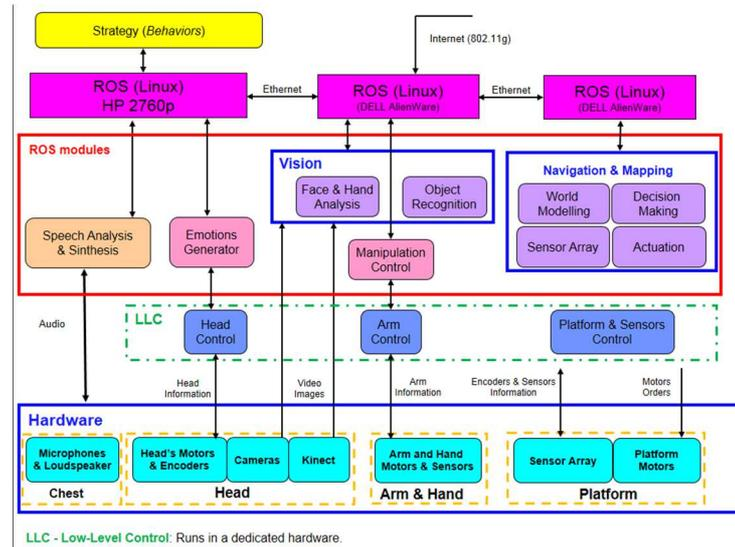
Figure 3. Modular organization of our software library. One Alienware notebook runs the Navigation and Mapping module, while the second Alienware notebook runs the Vision modules. The HP 2760p notebook runs Speech, Manipulation modules, high level processes and is the user interface thanks to the touch-screen capability.
